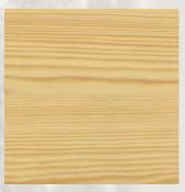
Pine is a softwood, with over 100 varieties. Pine trees are fast growing and sustainable. However, is not suitable for exterior work as it will rot quickly. Low grade Pine with lots of knots is used for frames in construction work, whilst high quality pine is used for furniture.
