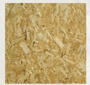
OSB or Oriented Strand Board is made from thin slices of wood, that are sorted to face the same direction. These are bonded with wax and glue. OSB is a very strong board, suitable for flooring or products requiring large panels.
