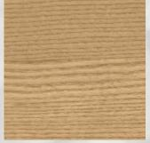
Ash is a hardwood that has over 50 varieties. The wood is characterised by a tight, straight, light coloured grain. It is very tough. Ash is used for interior furniture, but is less suitable for exterior projects as it is prone to rotting quickly.
