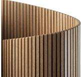
Similarto FlexiMDF, Flexi-wood is cut on both sides of the material to all the material to be curved. The deeper and more frequent the cuts, the tighter a curve can be created. Be careful, too many deep cuts, and the material will become very weak.
