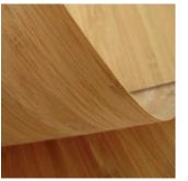
Veneers are thin slices of natural wood. These veneers are glued to the surface of manufactured boards to make them appear like a natural wood. Veneers can be easily cracked before they are glued. If they are not glued to the manufactured board well enough, they will peel away.
