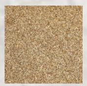
Sometimes called Particle Board, Chipboard is made from rough chips of wood and sawdust. This wood is then glued and compressed to create huge sheets. Chipboard is very inexpensive but is not particularly strong and will quickly dissolve when wet.
