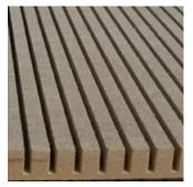
Flexi-MDF is made from normal MDF with the exception that it has grooves or channels cut on one face. This allows the MDF to have a gentle curved. The Flexi-MDF requires a frame to be constructed behind it to maintain the curve.
