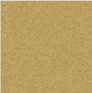
**MDF or Medium Density Fibreboard** is produced by breaking hardwoods and softwoods into small, short fibres. These fibres are glued together and heated and compressed to make large, incredibly strong sheets. Prolonged exposure to MDF dust is considered toxic. MDF will also dissolve with water.
