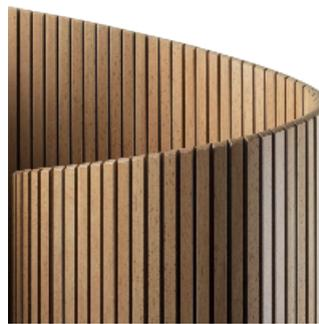
Similar to Flexi-MDF, Flexi-wood is cut on both sides of the material to all the material to be curved. The deeper and more frequent the cuts, the tighter a curve can be created. Be careful, too many deep cuts, and the material will become very weak.
