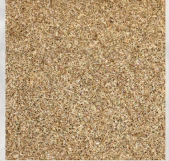
Sometimes called **Particle Board**, **Chipboard** is made from rough chips of wood and sawdust. This wood is then glued and compressed to create huge sheets. Chipboard is very inexpensive but is not particularly strong and will quickly dissolve when wet.
