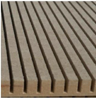
Flexi-MDF is made from normal MDF with the exception that it has grooves or channels cut on one face. This allows the MDF to have a gentle curve. The Flexi-MDF requires a frame to be constructed behind it to maintain the curve.
