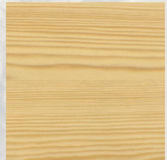
**Pine** is a softwood, with over 100 varieties. Pine trees are fast growing and sustainable. However, is not suitable for exterior work as it will rot quickly. Low grade Pine with lots of knots is used for frames in construction work, whilst high quality pine is used for furniture.
