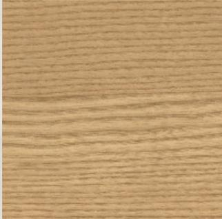
**Ash** is a hardwood that has over 50 varieties. The wood is characterised by a tight, straight, light coloured grain. It is very tough. Ash is used for interior furniture, but is less suitable for exterior projects as it is prone to rotting quickly.
