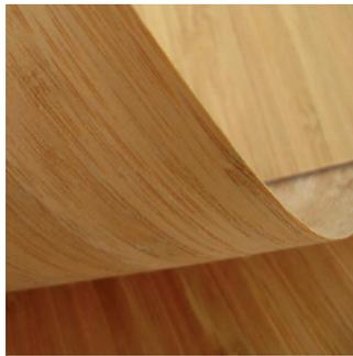
Veneers are thin slices of natural wood. These veneers are glued to the surface of manufactured boards to make them appear like a natural wood. Veneers can be easily cracked before they are glued. If they are not glued to the manufactured board well enough, they will peel away.
