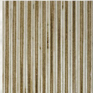
**Plywood** is a very popular board made from thin layers (ply) of natural wood. Each layer of wood is glued at 90° to the previous layer, making it rigid and strong. Plywood can be made from hardwood, softwood or both.
