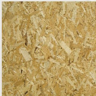
**OSB or Oriented Strand Board** is made from thin slices of wood, that are sorted to face the same direction. These are bonded with wax and glue. OSB is a very strong board, suitable for flooring or products requiring large panels.
