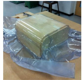
Flex-Ply is similar to regular plywood, with the exception that all layers are glued with the grain in the same direction. This allows the ply to bend along the grain. A vacuum press uses a heavy duty plastic bag and an air pump to bend a material such as flexi-ply around a foam pattern.
