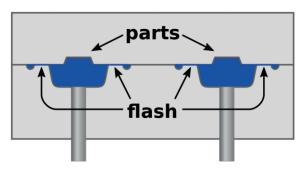
Compression moulding is a high-volume, high-pressure moulding method that is suitable for moulding complex, high-strength objects.
