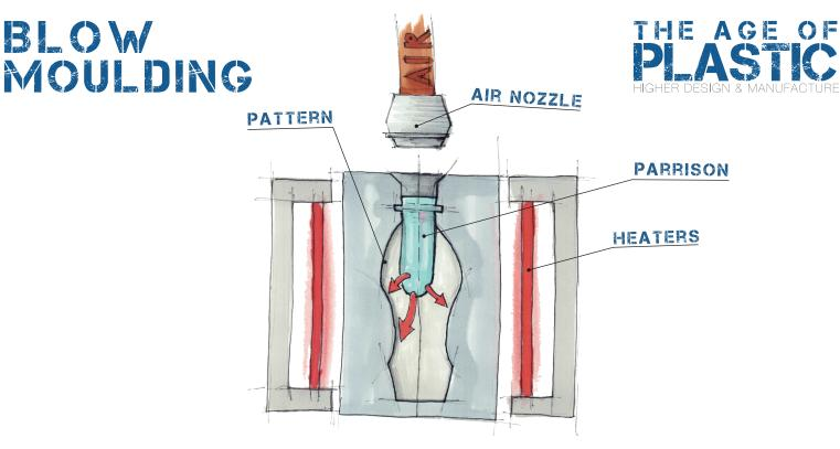
Blow molding is a manufacturing process that is used to create hollow plastic parts by inflating a heated plastic tube until it fills a mold and forms the desired shape.
