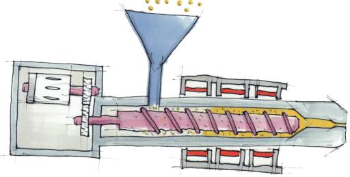
Along with Injection moulding, extrusion is a widely used method of forming plastics parts.
