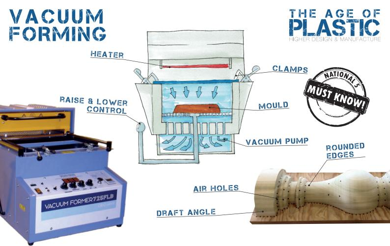
Vacuum forming is one of the oldest and most common methods of processing plastic materials.
