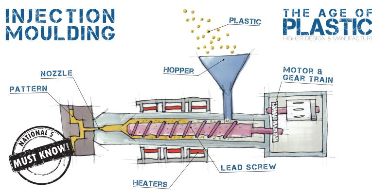
The plastic injection moulding process is a very quick way of producing high-quality, accurate parts.
