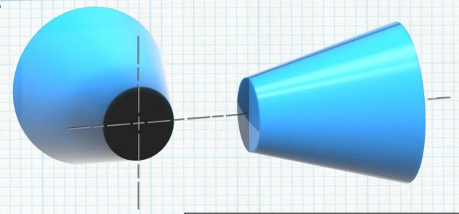
Create a manual orthographic drawing of the projection symbol
