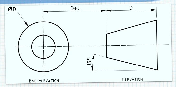
THE PROJECTION SYMBOL DEFINES WHAT TYPE OF ORTHOGRAPHIC PROJECTION IS BEING USED IN THE LAYOUT.
