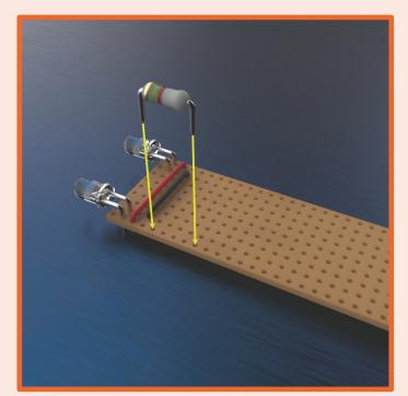
**13.** Time to stop the voltage frying those little LEDs. We do this by adding a resistor in series. Bend over the legs of the resistor and insert it into the holes. The direction of the resistor doesn't matter.
