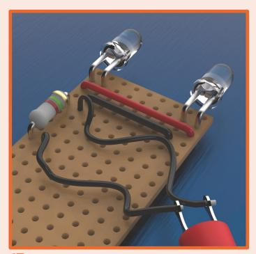
**15.** Insert in two BLACK wires for the switch, and solder these to your switch too. Solder these black wires to the board and again BREAK THE COPPER TRACK BETWEEN THESE WIRES!
