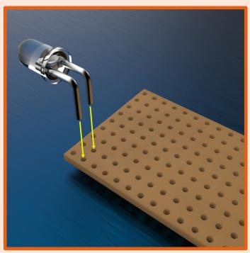
**2.** Fit the LED to the prototyping board.
