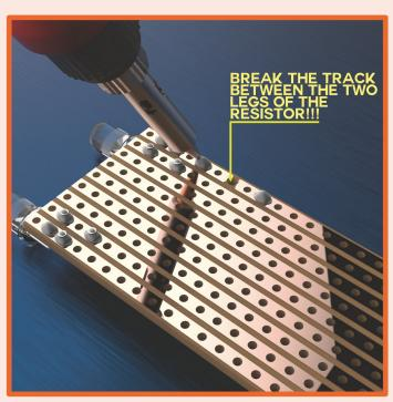
14. Okay, this is critical. Seriously. Stop. Solder the resistor to the board. Easy. Now... BREAK THE COPPER TRACK BETWEEN THE RESISTOR LEGS! OTHERWISE BAD THINGS HAPPEN TO THOSE LITTLE LEDs!
