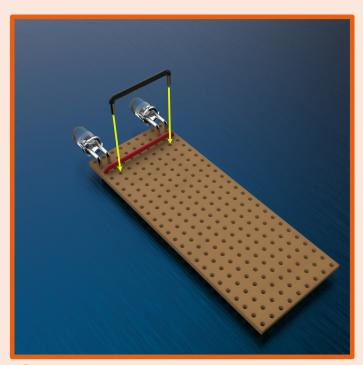
**10.** Next, the black wire. Bend over the ends at 90° using the pliers and insert into the inner holes.
