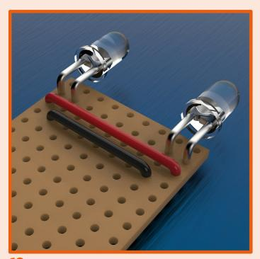
**12.** Check your wires are tidy and are secured to the prototype board.
