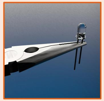
1. Grip your LED in a pair of needle-nosed pliers, leaving a small gap of a few millimetres. Bend the LED over 90°.
