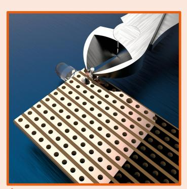
4. You should have excess wire sticking beyond the solder. This can cause a 'short circuit', so take your end-snip pliers and give your LED a hair-cut and remove the excess leg wire.
