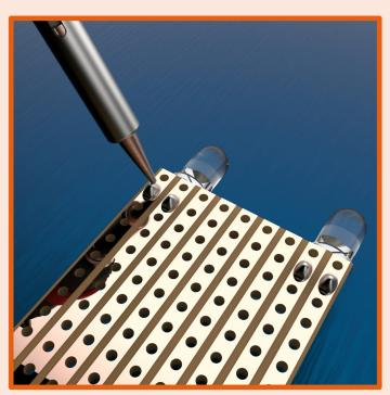
**6.** The soldering iron is used again to solder the LED to the prototyping board. Again, make sure you don't bridge between the tracks and accidentally create a short circuit.
