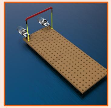
**9.** Time to wire things up. Take the RED wire and bend the ends over at 90° using the pliers.
