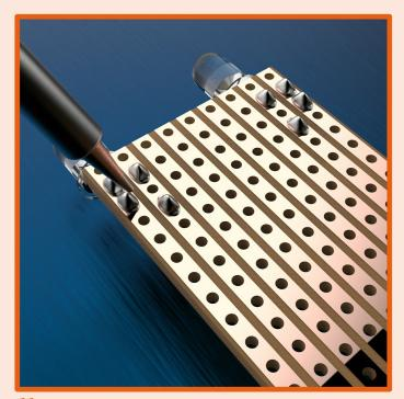
**11.** Flip your board over and solder the wires to the prototype board.
