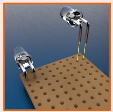
**5.** Take the second LED and use the needlenose pliers to bend at 90°. THE LONGER LEG **MUST** ALSO BE TO THE OUTSIDE OF THE BOARD! (this is very important...)
