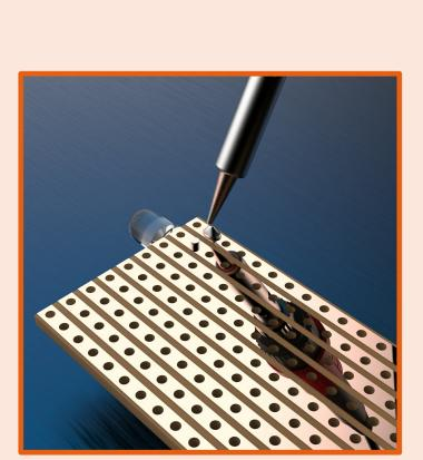
**3.** Grab your soldering iron (by the handle, not the hot bit) and solder the leg to the prototyping board. Make sure the solder doesn't 'bridge' between the two wires.
