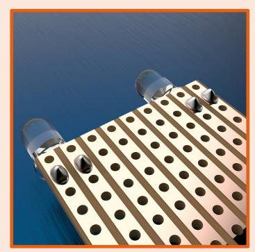
**7.** The end-snip pliers are used to trim the excess wire. Get the circuit looking nice and neat.
